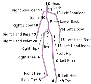
Fig. 1: 3D pose model. The names and numbering of the 21 joints in the pose follow the nomenclature in the ELMD dataset [23].
