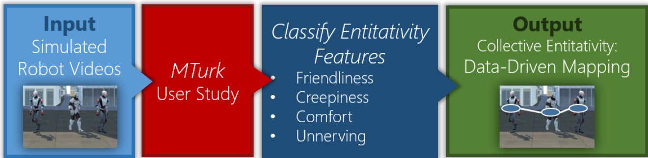
Fig. 3: We generate a variety of simulated robot groups using our motion model. Based on our precomputed EDM, we classify the entitativity of each cluster or group of pedestrians based on the four components: friendliness, creepiness, unnerving, and comfort.
